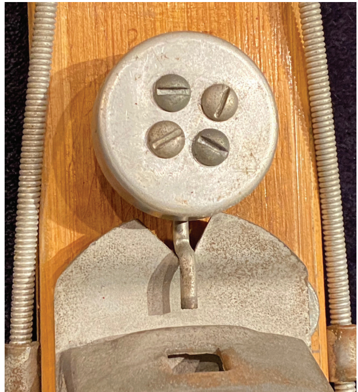
Stowe Binding – close up from above – The round housing holds a stiff wire spring. You can see the end of the spring as it comes out of the housing and fits into a notch on the plate.
