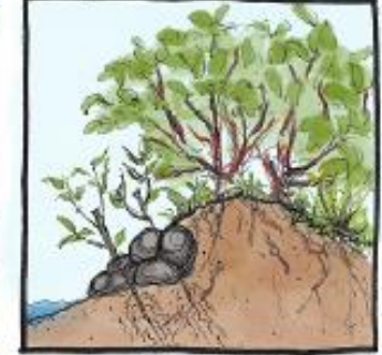
Leave berm, anchor with stone toe, plant live stakes and woody vegetation on berm.
