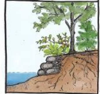
Leave and stabilize wall, backfill with gravel, plant robust native buffer.
