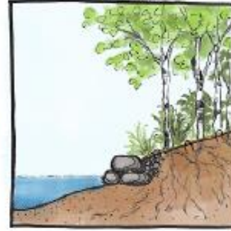
Remove top half of wall, regrade and slope back, backfill with gravel, plant.
