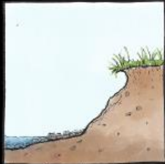
Steep, eroding, undercut bank
