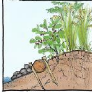
Regrade, slope berm back, stabilize bank & rock toe. Seed & plant woody species.
