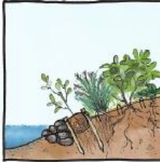
Remove wall or repurpose for rock toe, slope bank back, install fiber log, plant.
