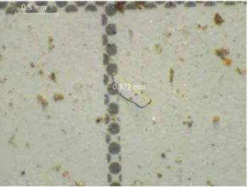
Figure 1: Examples of microplastics found from weekly samples at the Presumpscot River sample site.
