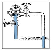
In this picture of an atmospheric vacuum breaker, a backsiphonage condition exists. This condition has caused the check-float to drop away from the air-inlet and seat on the check seat, which prevents the non-potable water from being backsiphoned. If the check-float did not seat properly, again only air would be sucked back into the domestic water system.
