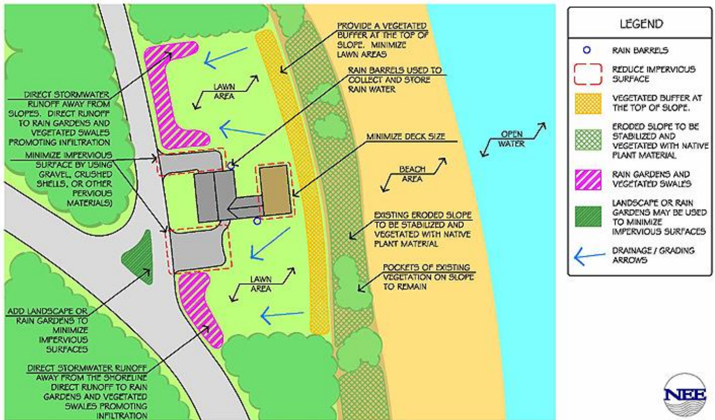
This figure demonstrates how a typical coastal property could be modified to reduce runoff and where appropriate runoff control techniques could be sited. (Graphic: New England Environmental, Inc.)
