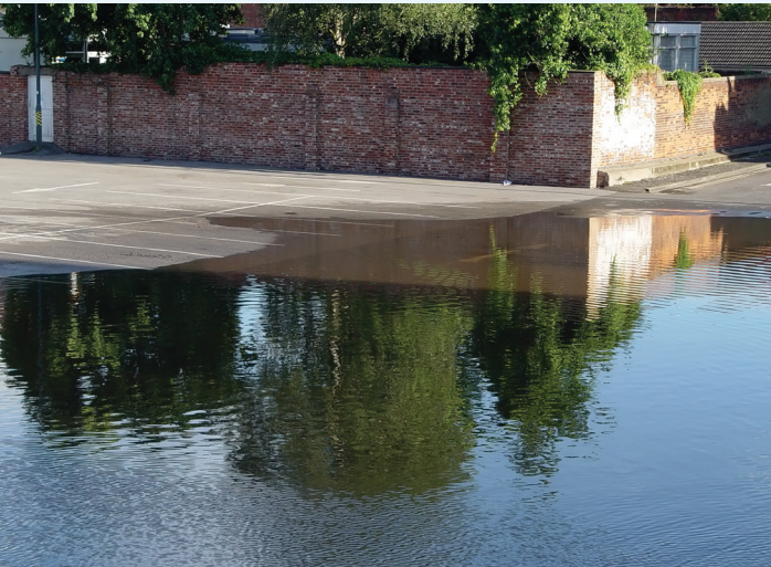
Parking lots are an example of an impervious surface: rain water cannot soak into the ground as it would naturally. To prevent the water from flooding into other areas, including the watershed, catch basins are required to hold and divert the water for treatment.
