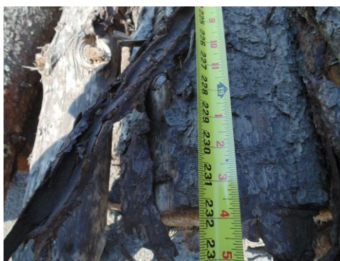
A 19 foot log. Any wood over 16'9" will cause issues while passing through the mill
