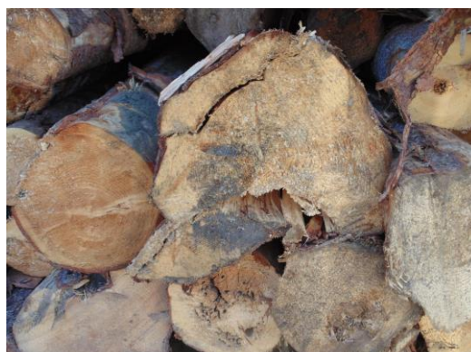
Shattered butt on a stick of tree length needs to be butted back to solid wood
