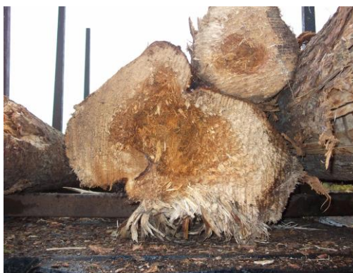
Spruce log with butt rot; rot is unacceptable.
